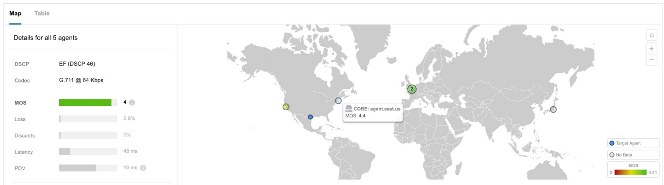
Figure 2: Voice quality scores such as MOS reflect the health of VoIP services across the globe
